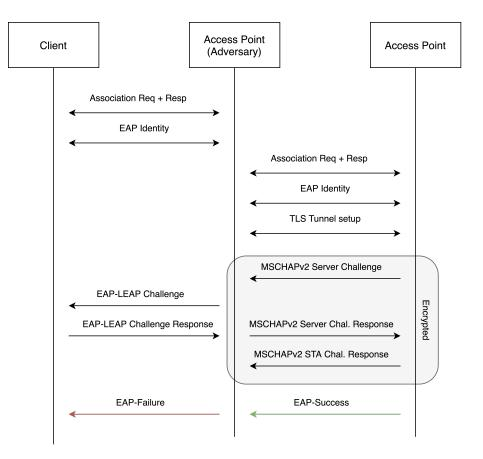
Figure 10: Flow diagram for the EAP-PEAP Relay attack
