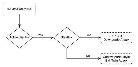
Figure 18: Attack flow diagram for WPA3-Enterprise
