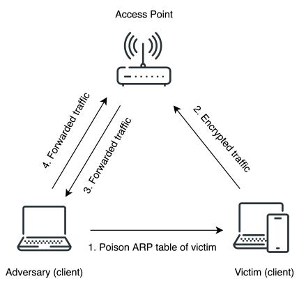
Figure 12: Flow diagram for the Hole196 vulnerability
