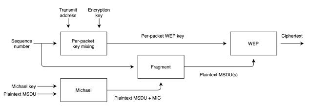
Figure 5: Temporal Key Integrity Protocol diagram
