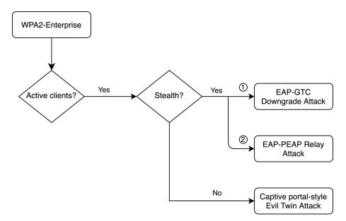
Figure 16: Attack flow diagram for WPA2-Enterprise
