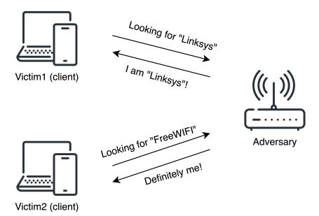
Figure 11: Flow diagram for the KARMA attack
