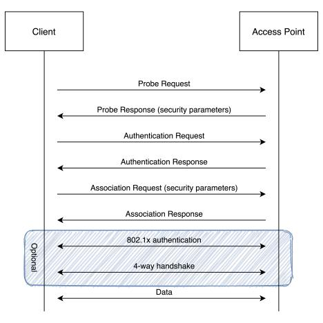
Figure 1: Wi-Fi connection phases
