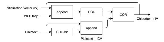
Figure 3: WEP RC4 encryption algorithm
